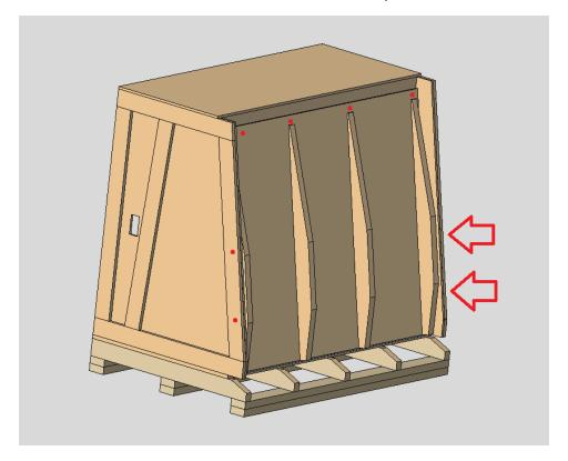
NOTE: Before lowering the handle, be sure to place a towel or other soft material over the door hinge area of the crate to prevent scratches or other damage to the handle.
